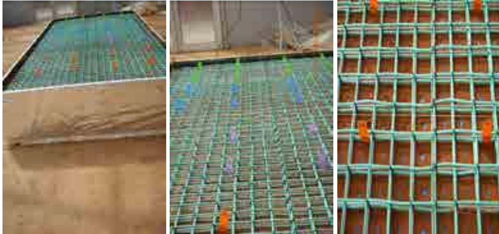
Figure 5.1 The grid used to heat soil with a computer program in containers (a – c).
